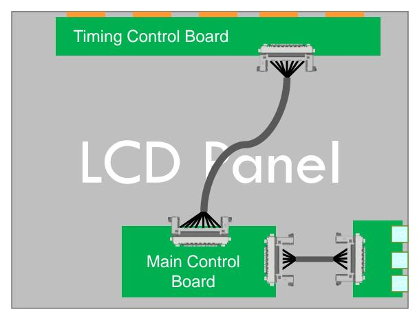
Simple diagram of a possible usage of an FI-R connector inside a display.
