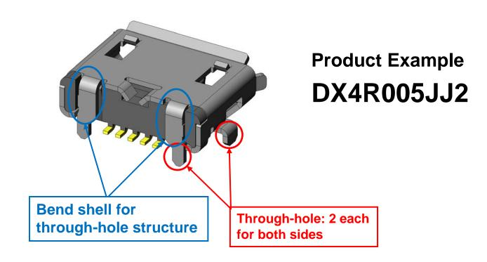
The on-board through-hole type is durable against impact when plug is inserted.
