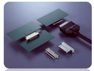
(dock) plug which can be mounted directly to a PCB. An outer metal shell acts as a mechanical key and guide during mating, and also helps minimize EMI. Locking latches are included on the cable plug to ensure secure mating, while large guide posts on the cradle plug allow for blind mating/docking.
